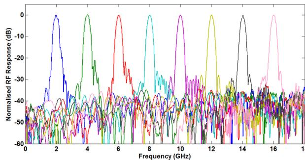
Figure 3: Tuned RF responses of the microwave photonic filter [2].
