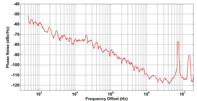
Figure 6: Phase noise response of the OEO signal.
