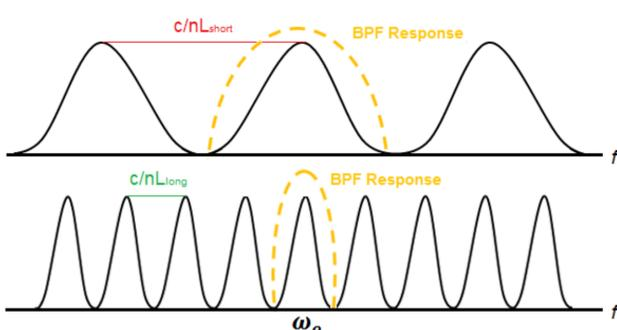
Figure 1: Operating principle of a short and long loop OEO, showing the BPF requirement for single-mode oscillation.
