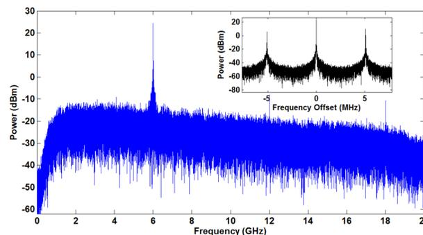
Figure 4: Measured spectrum of a 6 GHz oscillation, with a zoom-in view of the fundamental mode inset.
