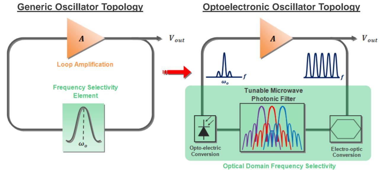
Figure 2: Schematic diagram of a generic oscillator and the optoelectronic oscillator design.
