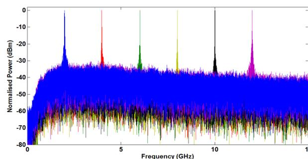
Figure 5: Normalised OEO spectra tuned over a frequency range of 0 to 14 GHz
