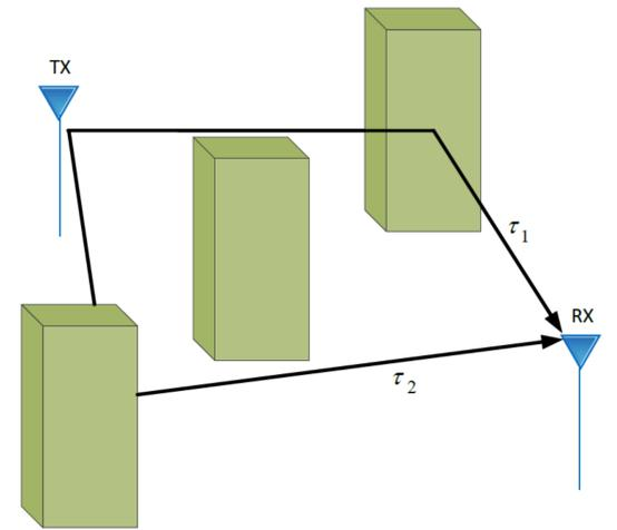
Fig.2: Multipath Propagation for impenetrable scenario.
