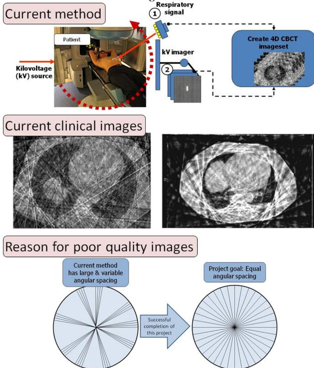
**Figure 2. Top:** in the current 4D CBCT method there is no feedback of the respiratory signal to the imaging system. **Middle:** this limitation causes streak artefacts in clinical images. **Bottom:** the reason for poor quality clinical images<sup>10, 11</sup> is large angular spacing between projections with fixed rotation speed (left). The solution is to obtain equispaced projections by the proposed RM 4D CBCT (right).
