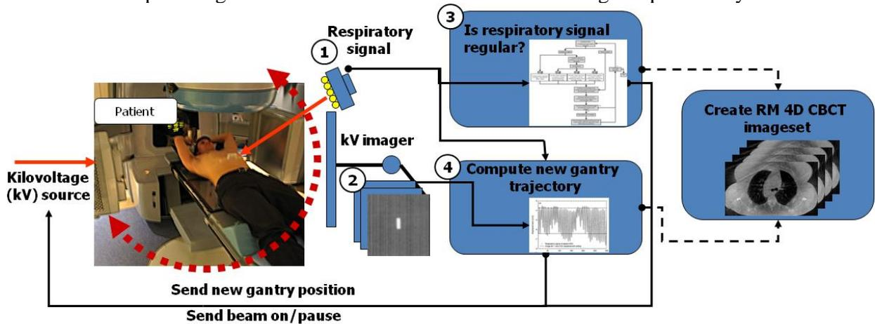
**Figure 3.** A schematic of the proposed RM 4D CBCT method in which the respiratory signal is actively used to modulate gantry rotation and image acquisition.
