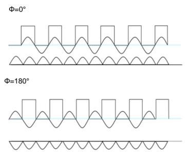
Fig 4. Phase-sensitive Demodulation
